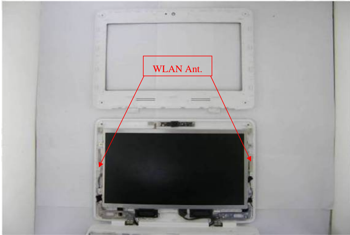
Internal View of EUT – 9 (WLAN Module)
