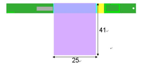
Figure 1. RTL8188CUs Slim Module Mechanical Specification
