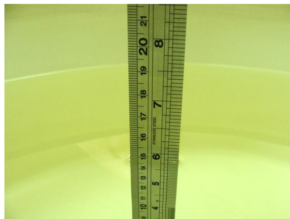
Fig 6.2 Photo of Liquid Height for Body SAR
