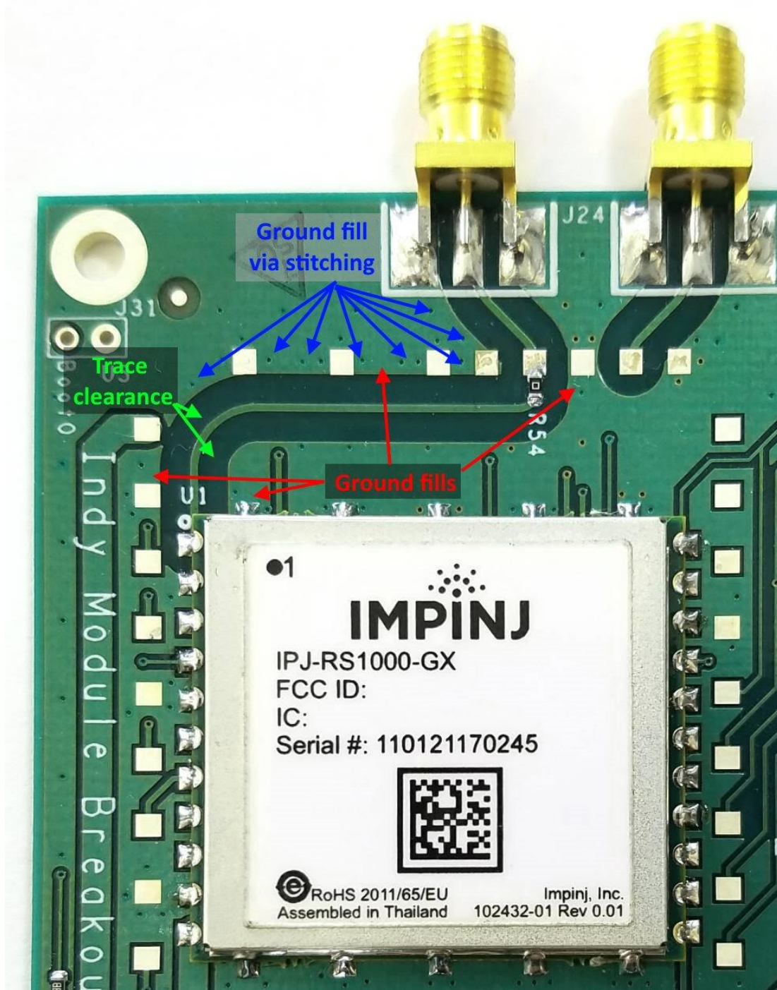
Figure 4 – RS1000 RF PCB Layout Example – Indy Module Breakout Board
