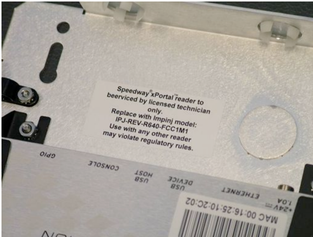
Close up of label that indicates the transmitter can only be replaced with a specific SKU
