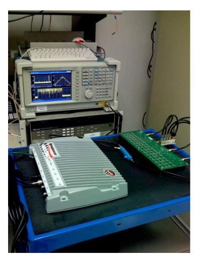
The reader is started to perform RFID tag inventory and a PC program controls the RSA3303A via GPIB in order to automate the exact measurements of 20 captures per channel. The measurements taken are:
