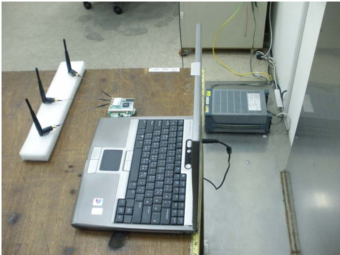
Photo 2: Conducted Emission Test Set-up photo
