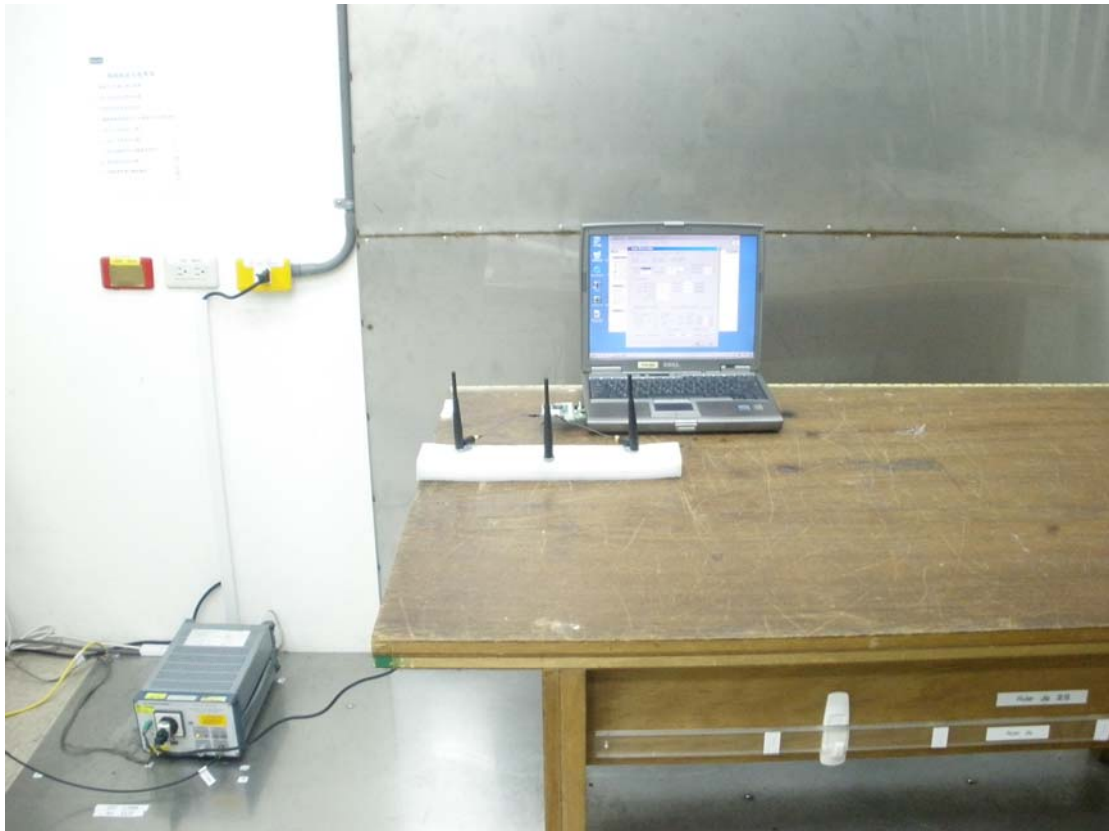
Photo 1: Conducted Emission Test Set-up photo
