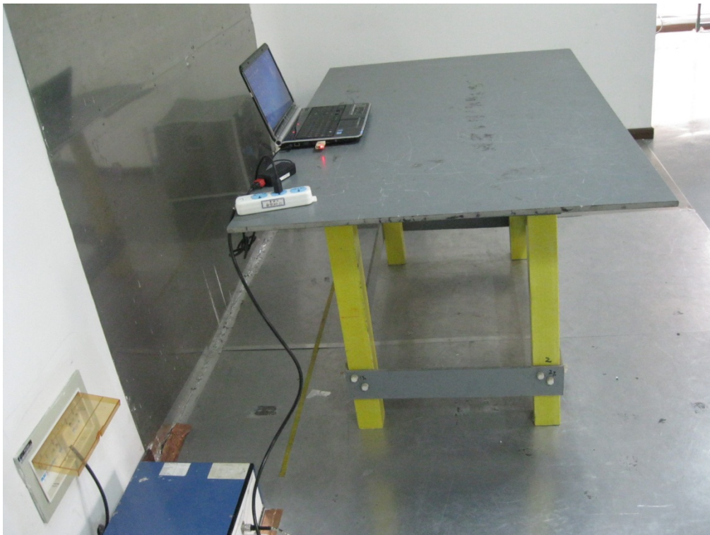
Conducted Emissions Test Setup - Side View
