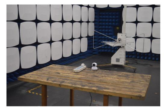
3. Radiated Field Strength Measurement(30MHz-1GHz)
