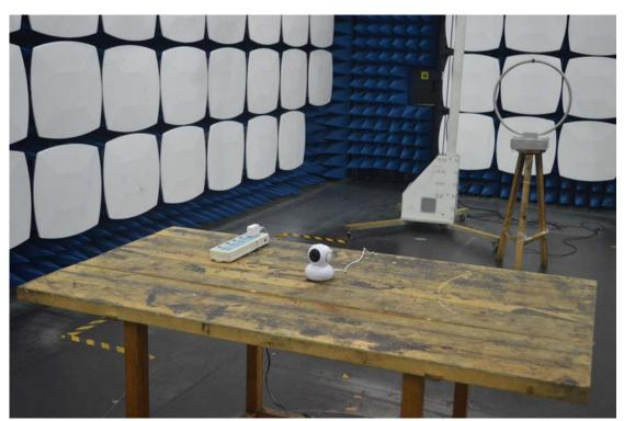
3. Radiated emission (9KHz-30MHz)
