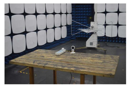
4. Radiated Field Strength Measurement(above 1GHz)
