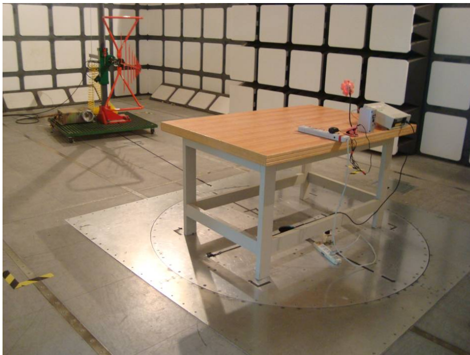
Radiated Emissions - Rear View (Below 1 GHz)
