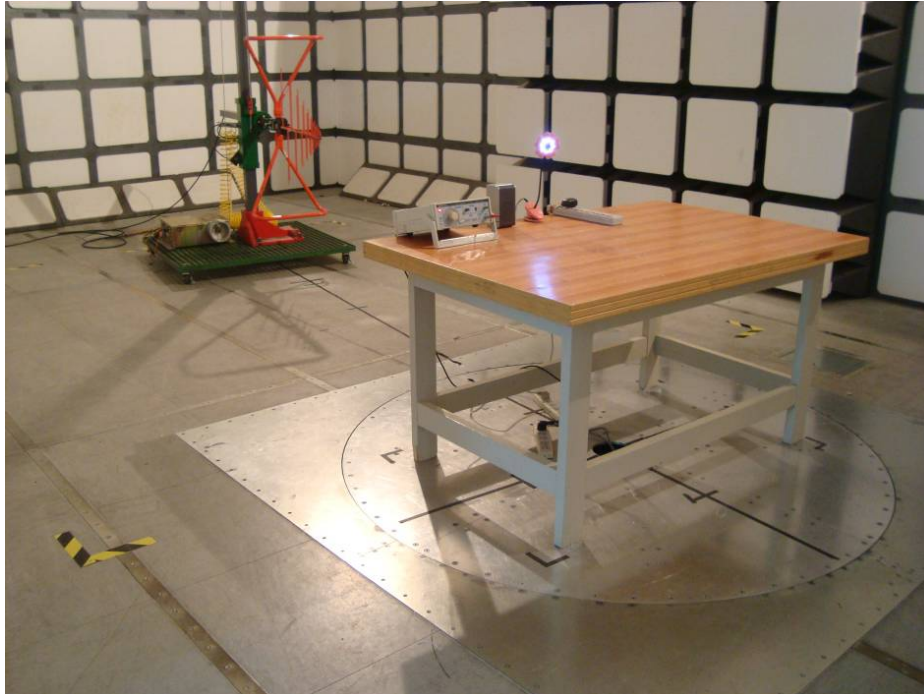
Radiated Emissions - Rear View (Below 1 GHz)
