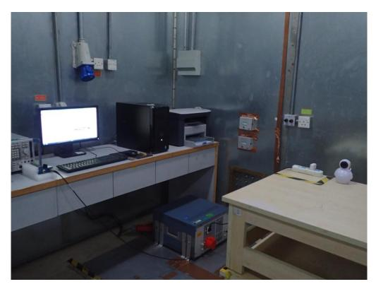
RADIATED EMISSION TEST SETUP BELOW 1GHZ
