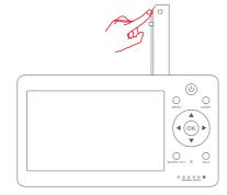
2.2.2. Plug an end of the charging cable into the USB socket in the side of the monitor. Plug another end into the power adapter. Then plug the adapter into a power socket.
