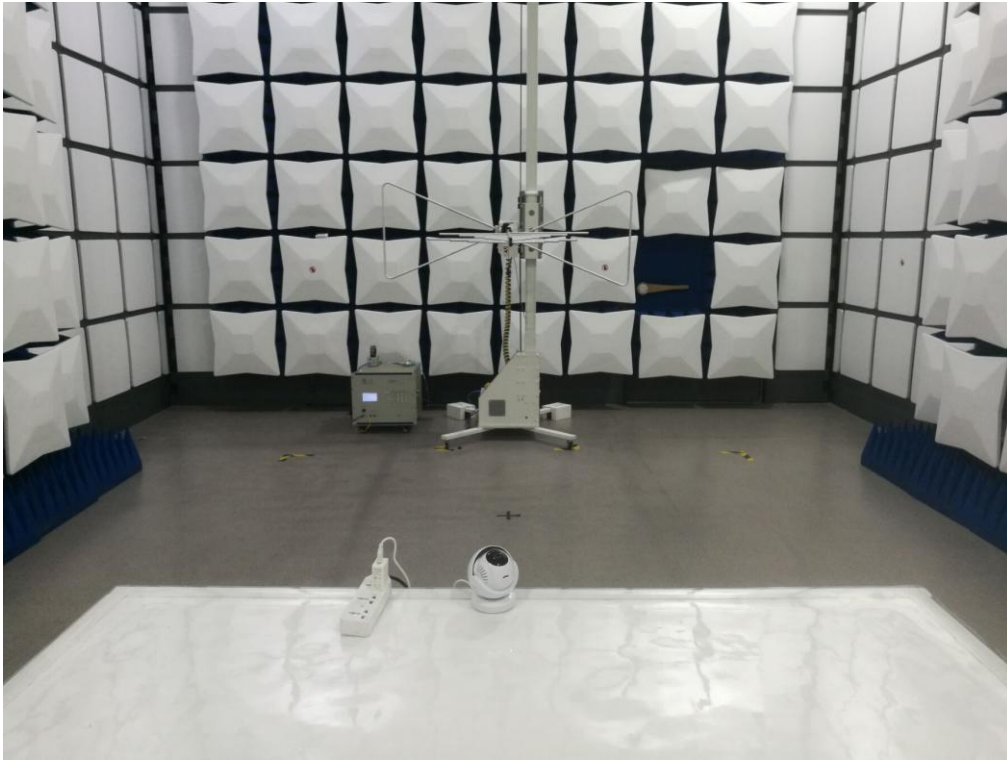
FCC RADIATED EMISSION TEST SETUP ABOVE 1GHZ
