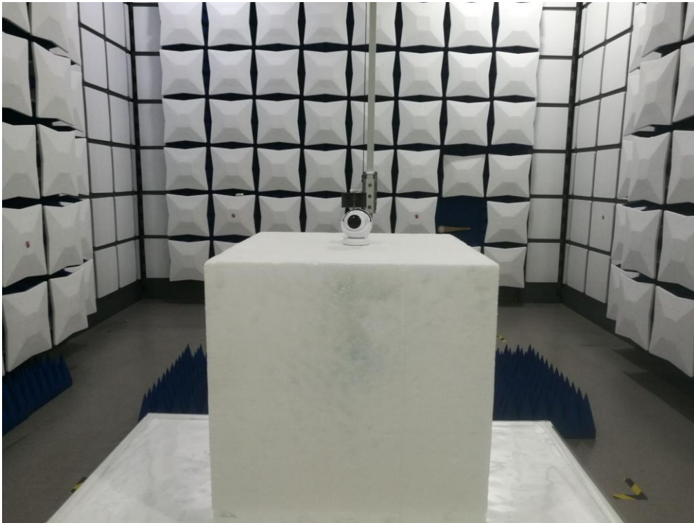
FCC RADIATED EMISSION TEST SETUP ABOVE 1GHZ
