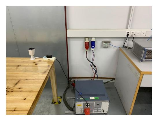
FCC RADIATED EMISSION TEST SETUP
