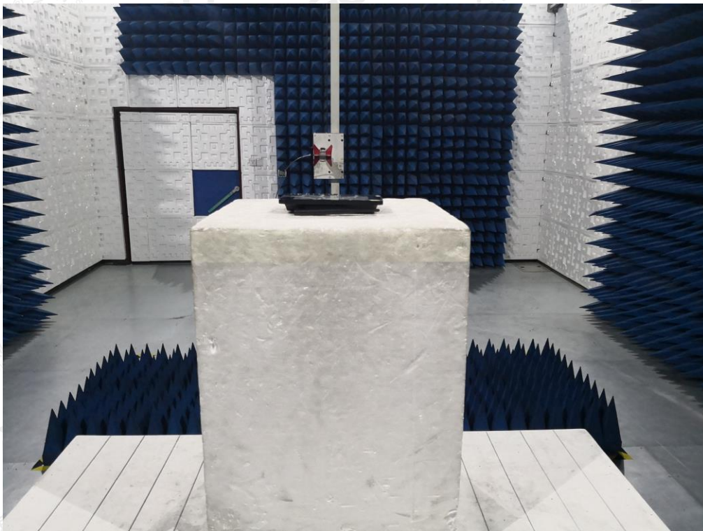
FCC RADIATED EMISSION TEST SETUP ABOVE 1GHZ
