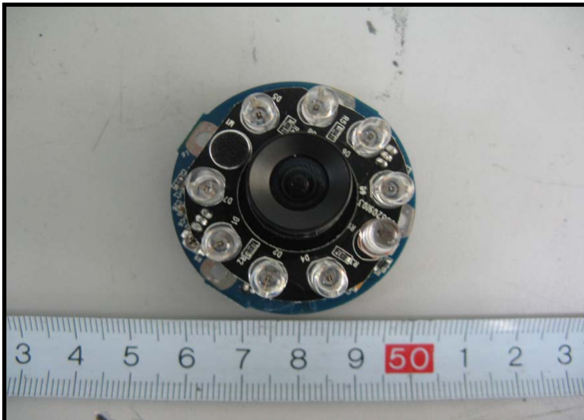
EUT-Camera Board Components View
