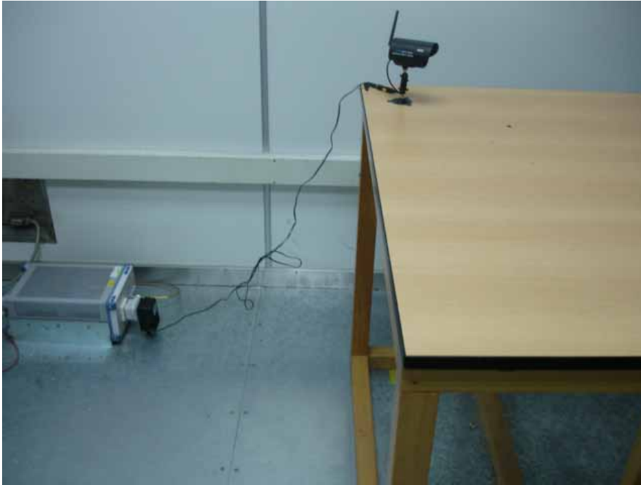
Photo 2 Radiated Emission Test
