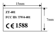
The Label must not be a stick-on paper label. The Label on these products must be permanently affixed to the product and readily visible at the time of purchase and must last the expected lifetime of the equipment not be readily detachable.
