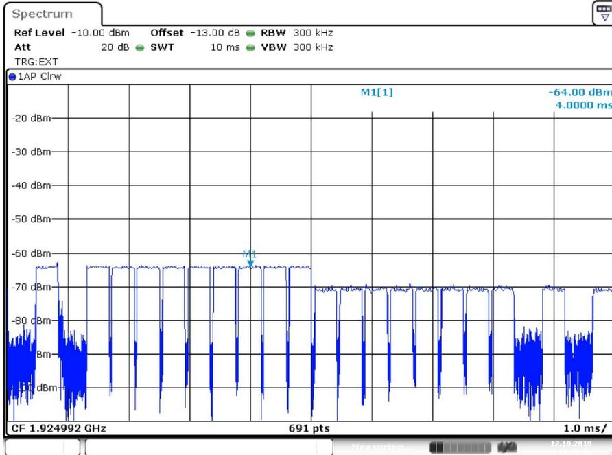
**8.3.2 c) Transmission on interference-free receive time window**
