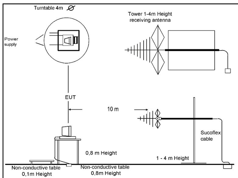
**1GHz – 10 GHz:****Test Set-up 5:**
