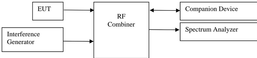
This test setup is used for all Monitoring and Time and Spectrum Access Procedure tests. The path loss from the signal generator to the EUT is measured with a power meter before the testing is started.
