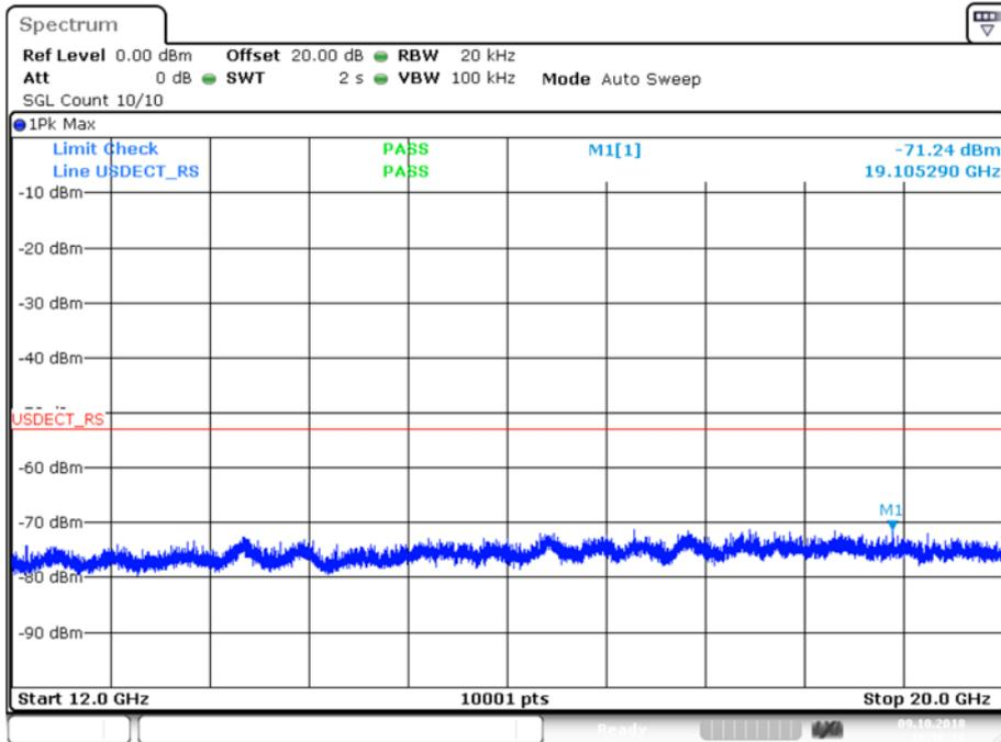
Receiver Spurious Emissions, Conducted, 12 GHz – 20 GHz
