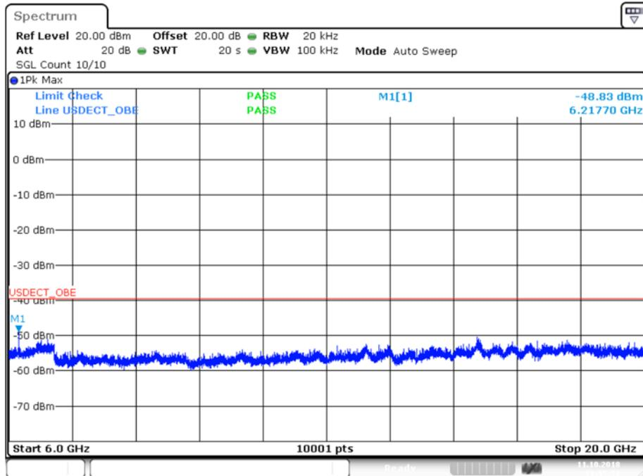
The BS spurious out-of-band transmission level is below the indicated limit.
