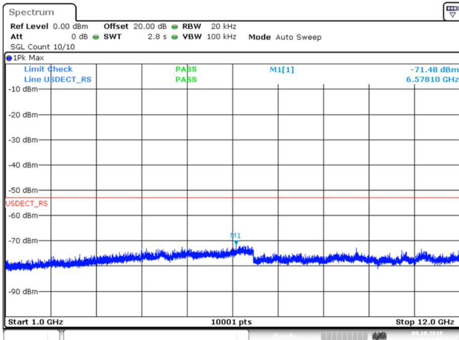
**Receiver Spurious Emissions, Conducted, 1 GHz – 12 GHz**
