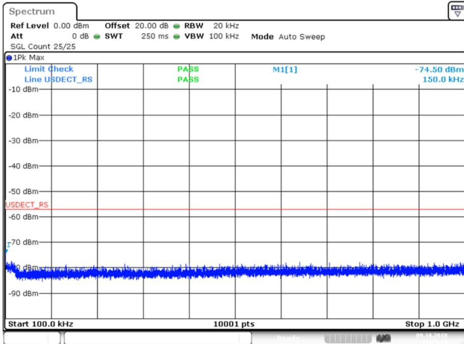
**Receiver Spurious Emissions, Conducted, 100 kHz – 1 GHz**
