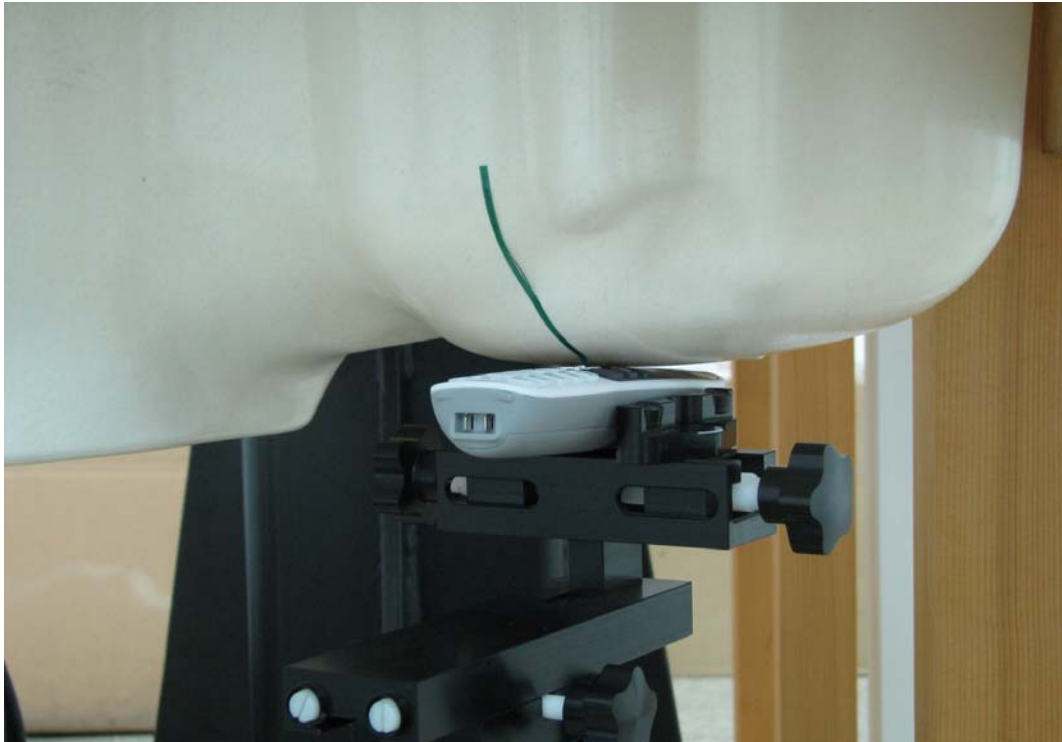
Measurement Position of Right-Cheek (RC) with Handset
