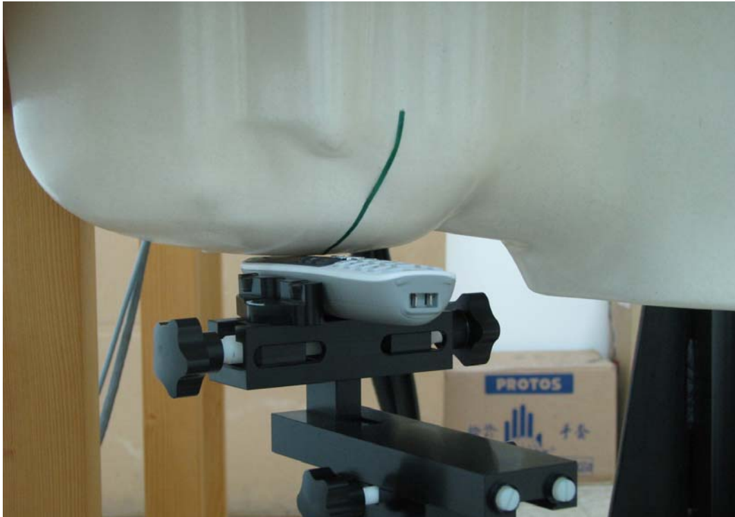
Measurement Position of Left-Cheek (LC) with Handset
