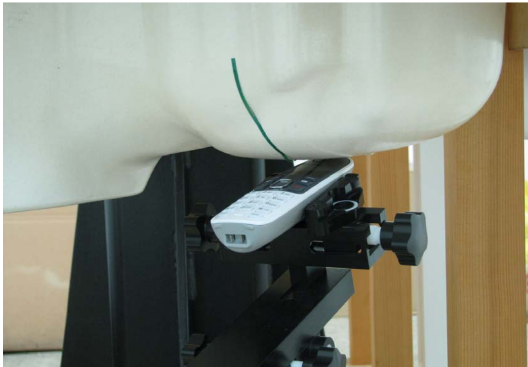
Measurement Position of Right-Tilt (RT) with Handset
