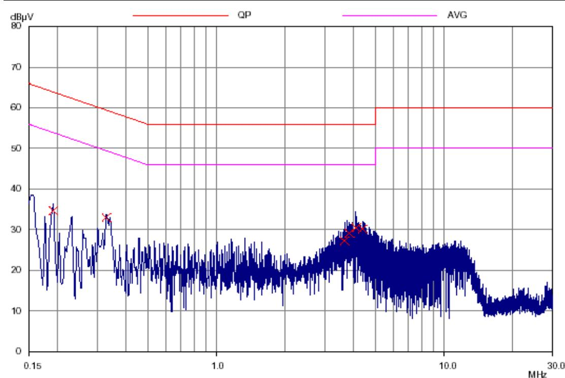
**Model No.: A490 / Adaptor 1**Operation Mode : Base ChargingNeutralTest Date : Nov. 22, 2009Temperature : 20 °CHumidity : 72 %
