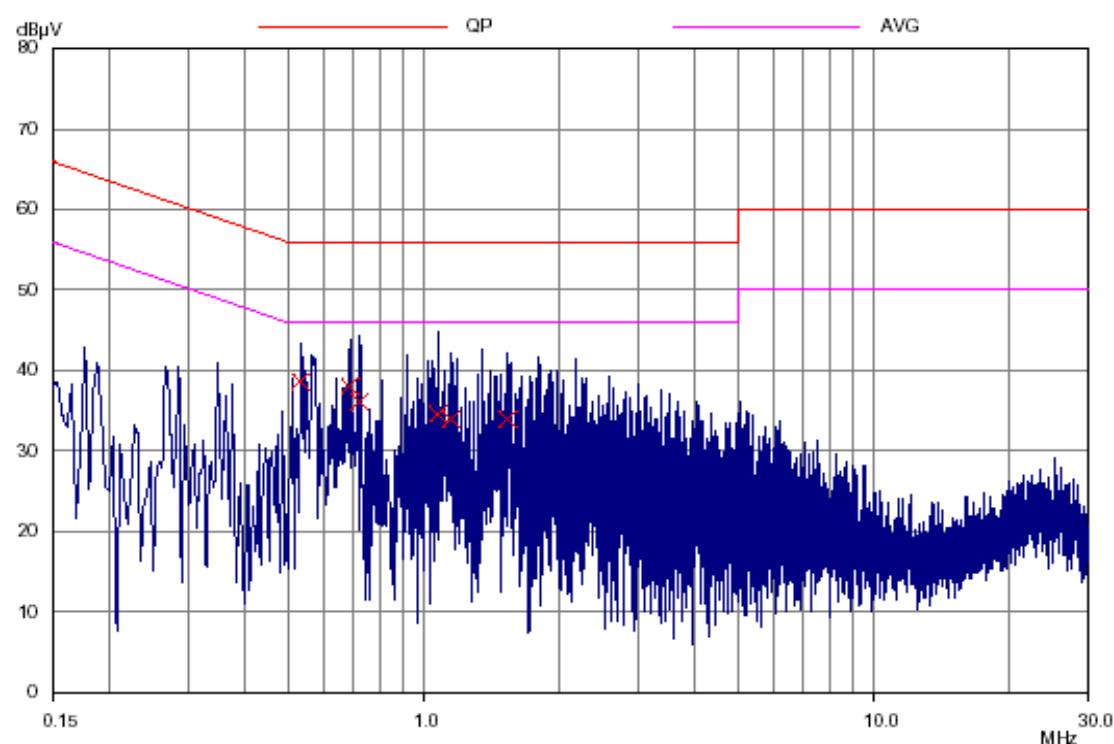
**Model No.: A495 / Adaptor 2**Operation Mode : Base ChargingNeutralTest Date : Nov. 22, 2009Temperature : 20 °CHumidity : 72 %
