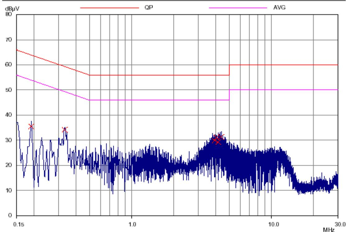
**Model No.: A495 / Adaptor 1**Operation Mode : Base ChargingNeutralTest Date : Nov. 22, 2009Temperature : 20 °CHumidity : 72 %
