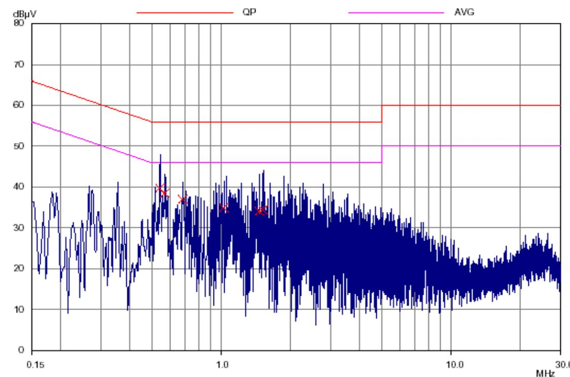
**Model No.: A490 / Adaptor 2**Operation Mode : Base ChargingNeutralTest Date : Nov. 22, 2009Temperature : 20 °CHumidity : 72 %
