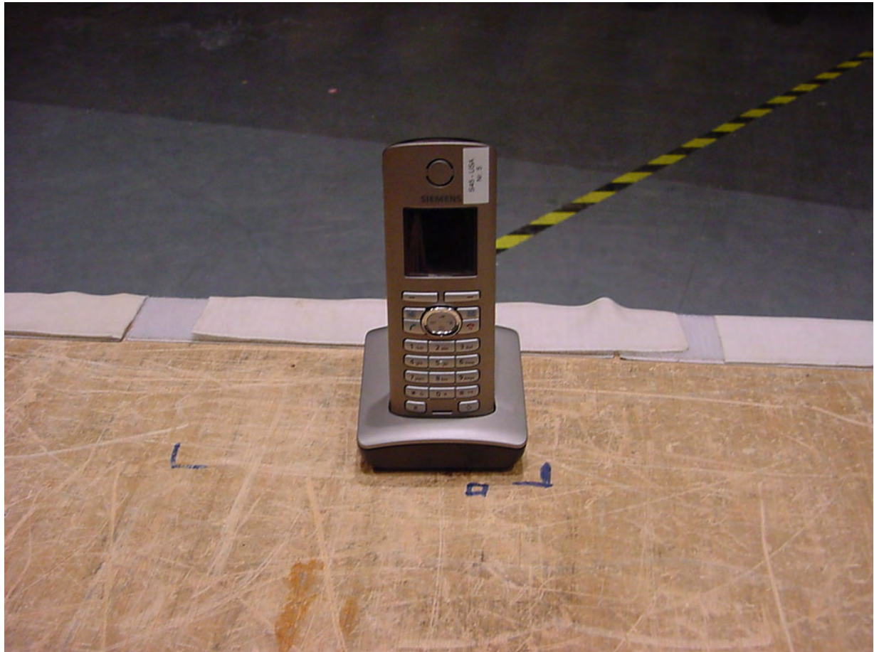
Photo 1: Radiated Emissions S45
