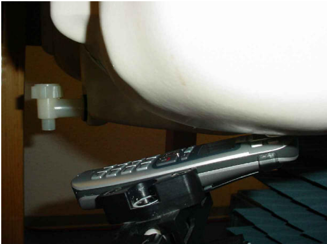
Photo 12: Test position left hand tilted 15°
