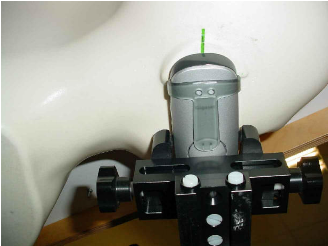
Photo 16: Test position right hand tilted 15°
