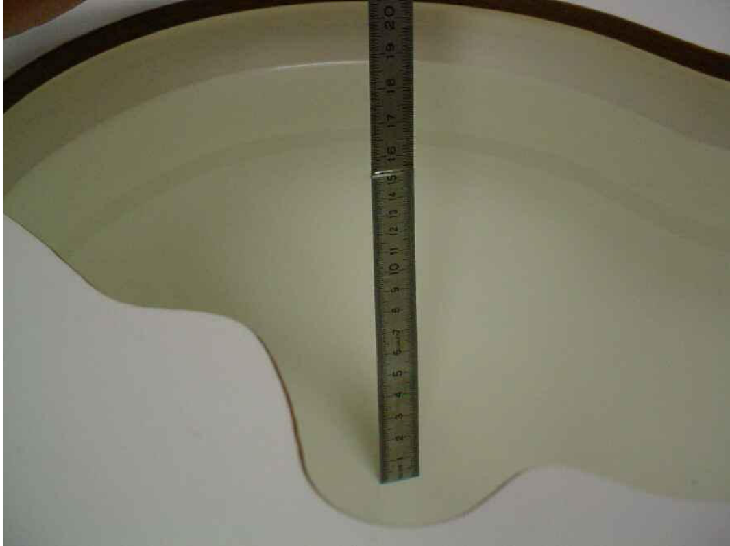
Photo 23: Liquid depth 1900 MHz body simulating liquid
