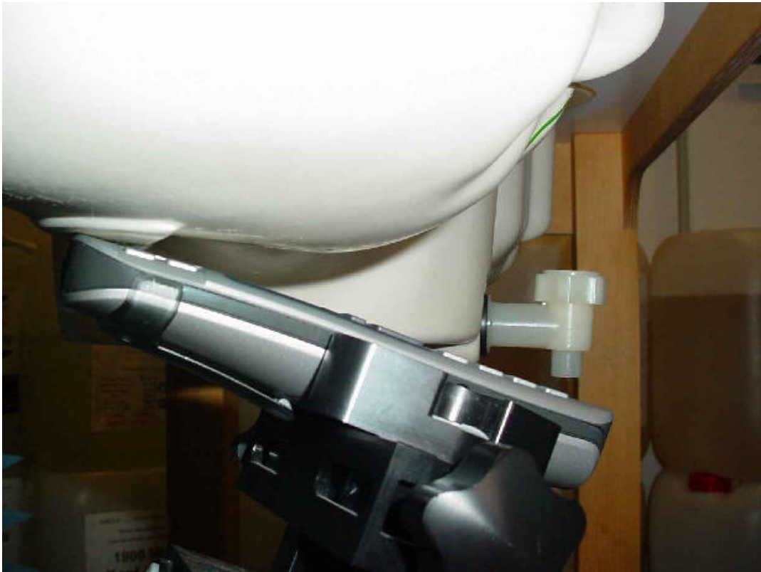
Photo 18: Test position body worn front side without any distance
