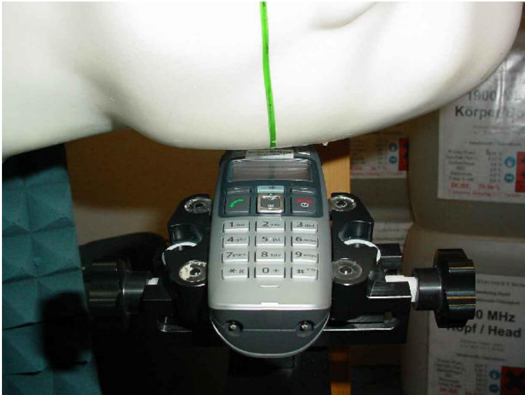
Photo 12: Test position left hand tilted 15°
