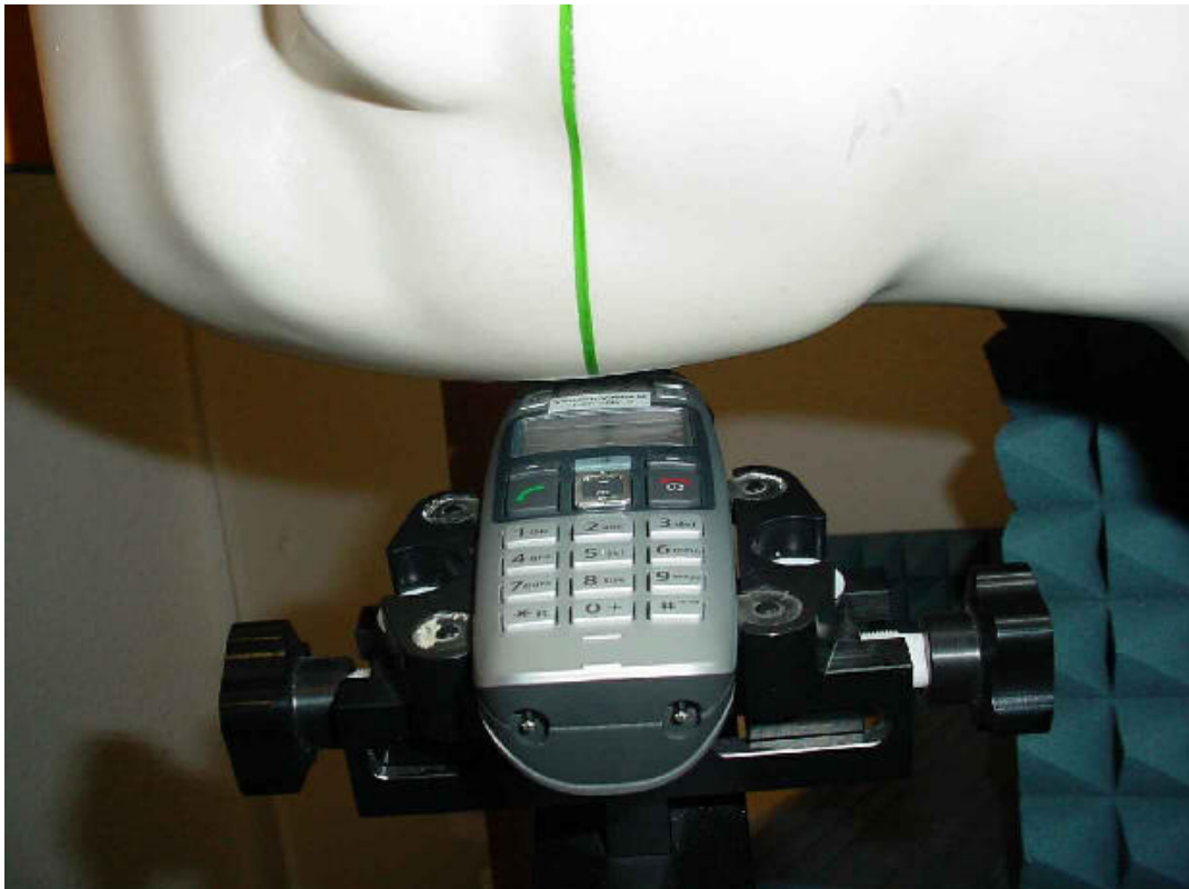
Photo 16: Test position right hand tilted 15°
