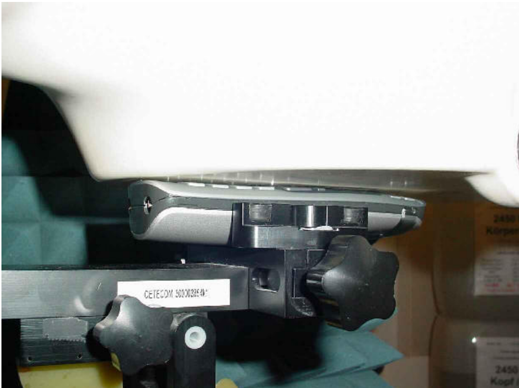
Photo 18: Test position body worn front side without any distance
