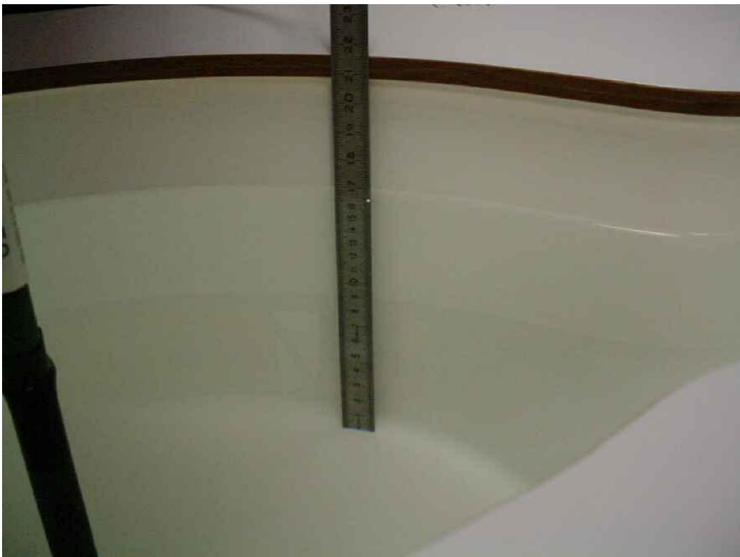
Photo 23: Liquid depth 1900 MHz body simulating liquid
