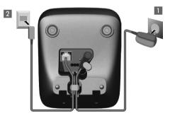
◆ Only use the power adapter and phone cord **supplied**. Pin connections on telephone cables can vary (pin connections → page 48).
