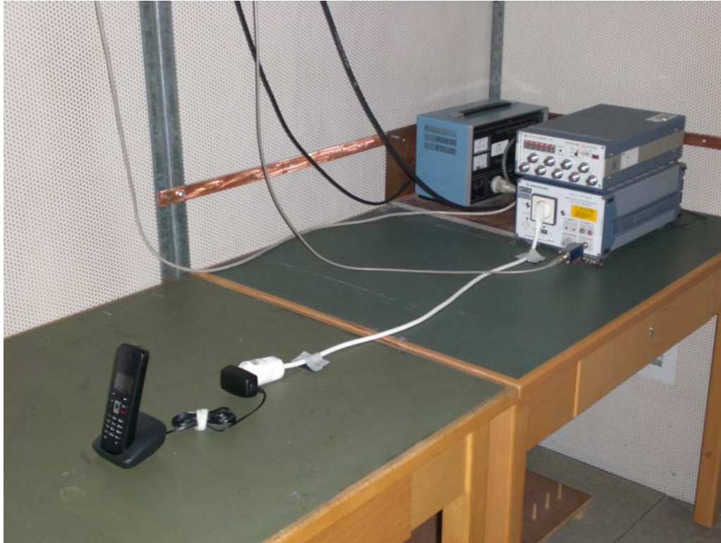
Photo 1: Power Line Conducted Emission Test
