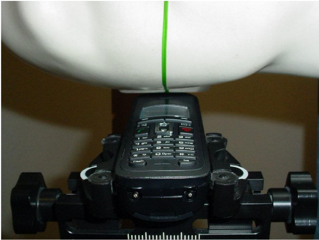
Photo 16: Test position right hand tilted 15°
