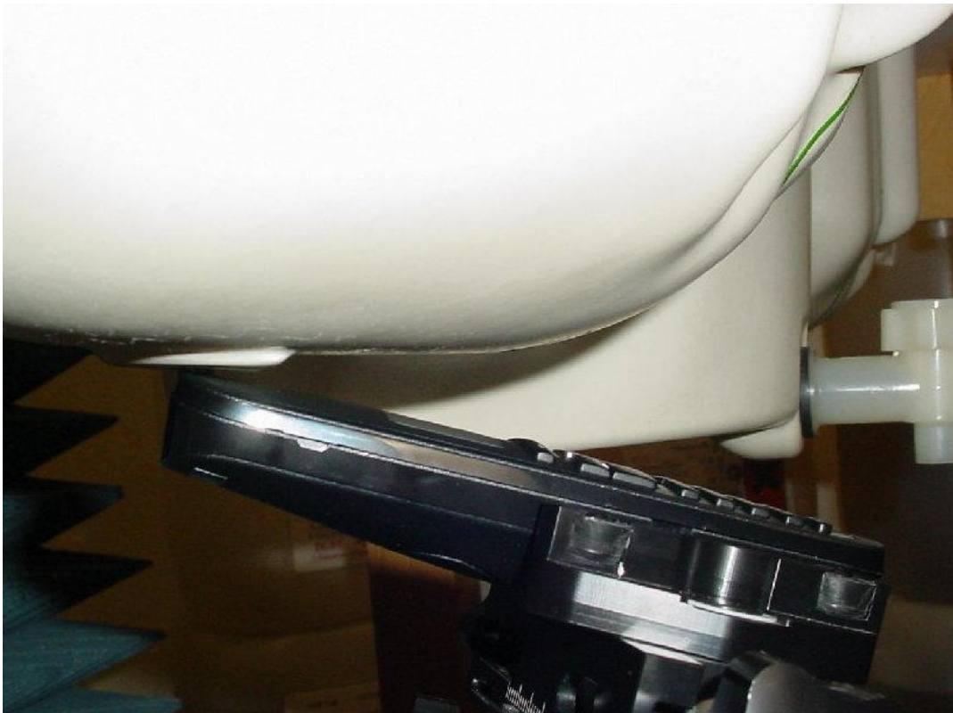
Photo 16: Test position right hand tilted 15°
