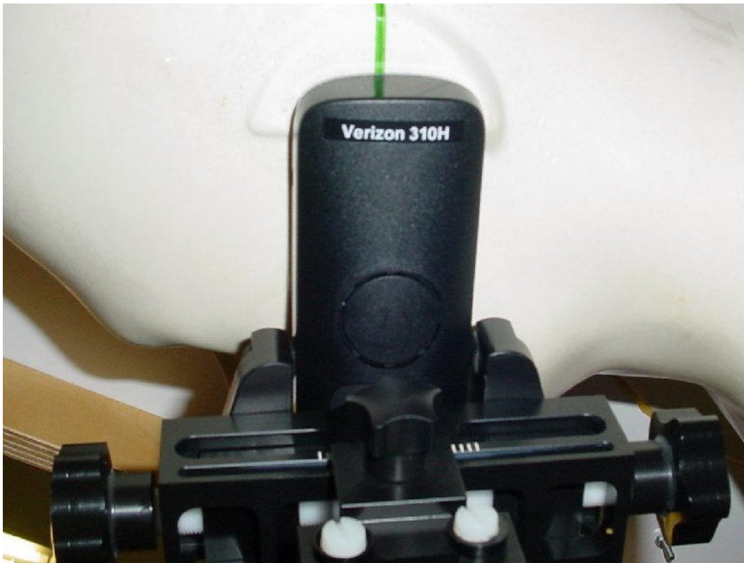
Photo 10: Test position left hand tilted 15°
