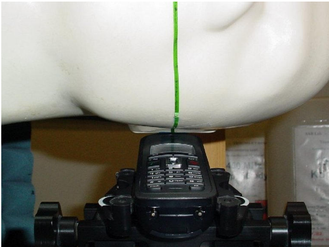
Photo 10: Test position left hand tilted 15°
