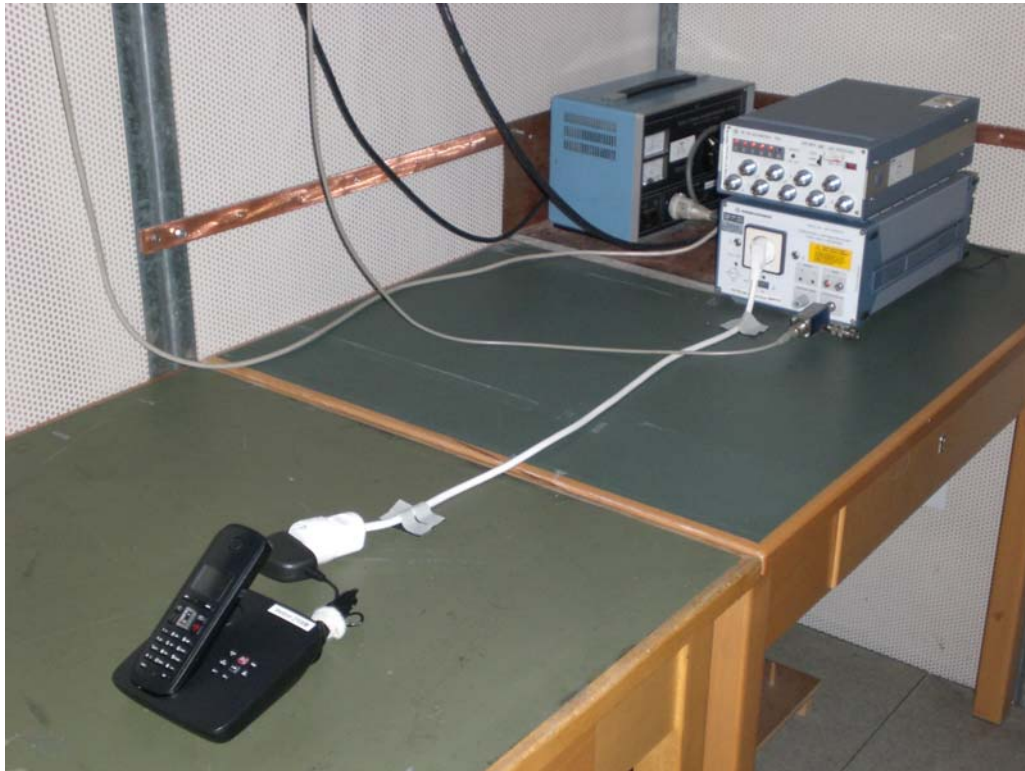
Photo 1: Power Line Conducted Emission Test
