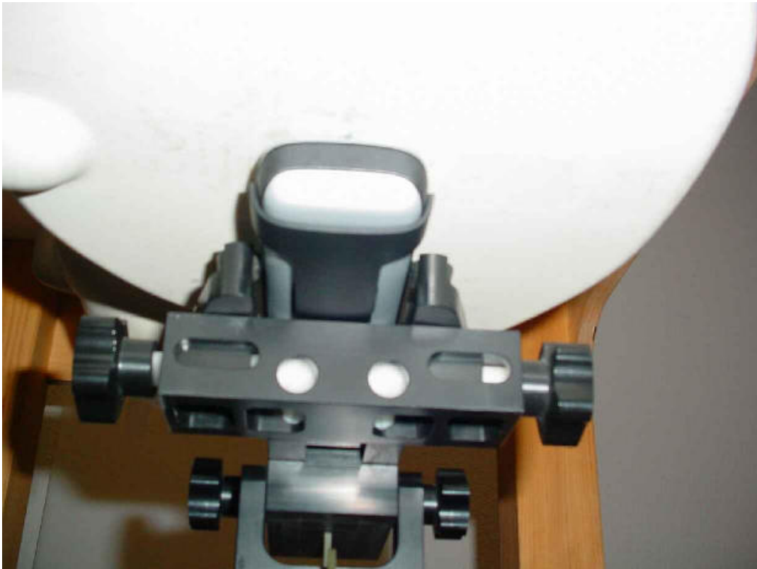
Photo 20: Test position body worn rear side without any distance
