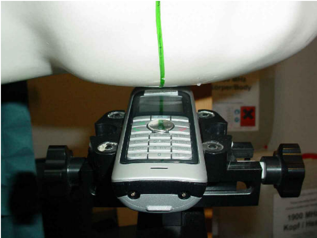
Photo 12: Test position left hand tilted 15°
