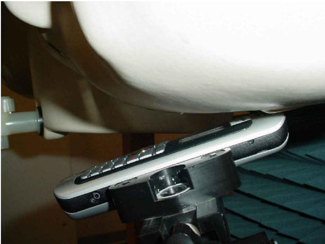
Photo 12: Test position left hand tilted 15°
