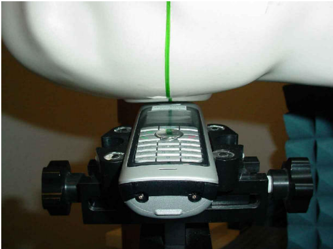
Photo 16: Test position right hand tilted 15°
