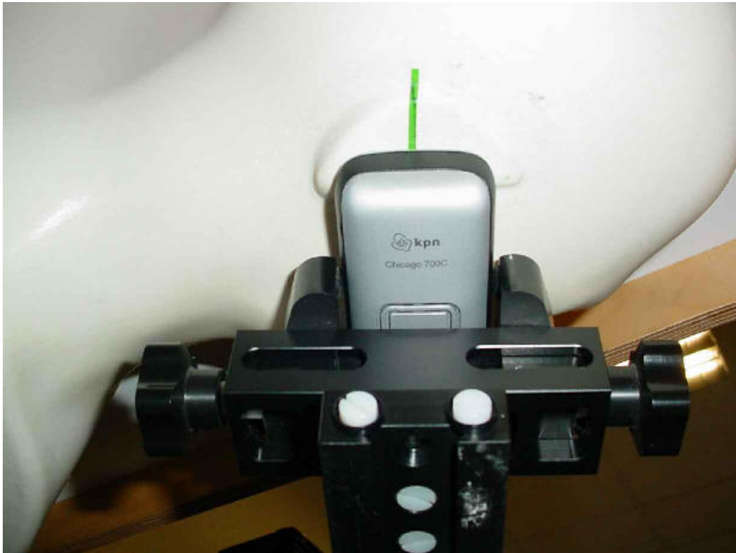
Photo 16: Test position right hand tilted 15°
