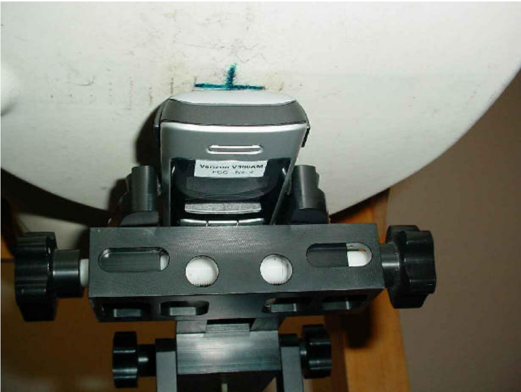
Photo 21: Test position body worn rear side without any distance
