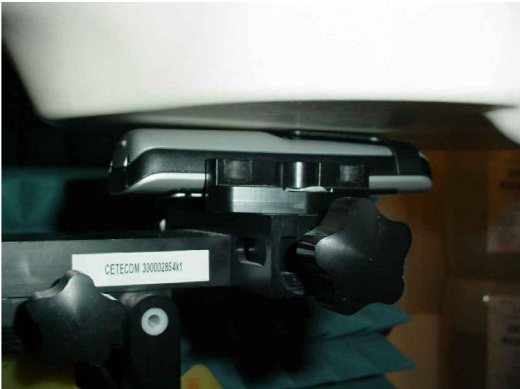
Photo 20: Test position body worn rear side without any distance
