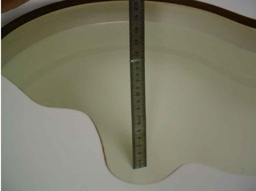
Photo 23: Liquid depth 1900 MHz body simulating liquid
