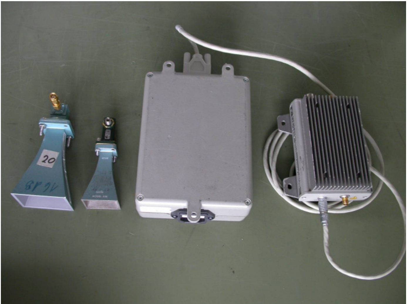
Equipment for spurious emission measurement from 12 GHz to 27 GHz
