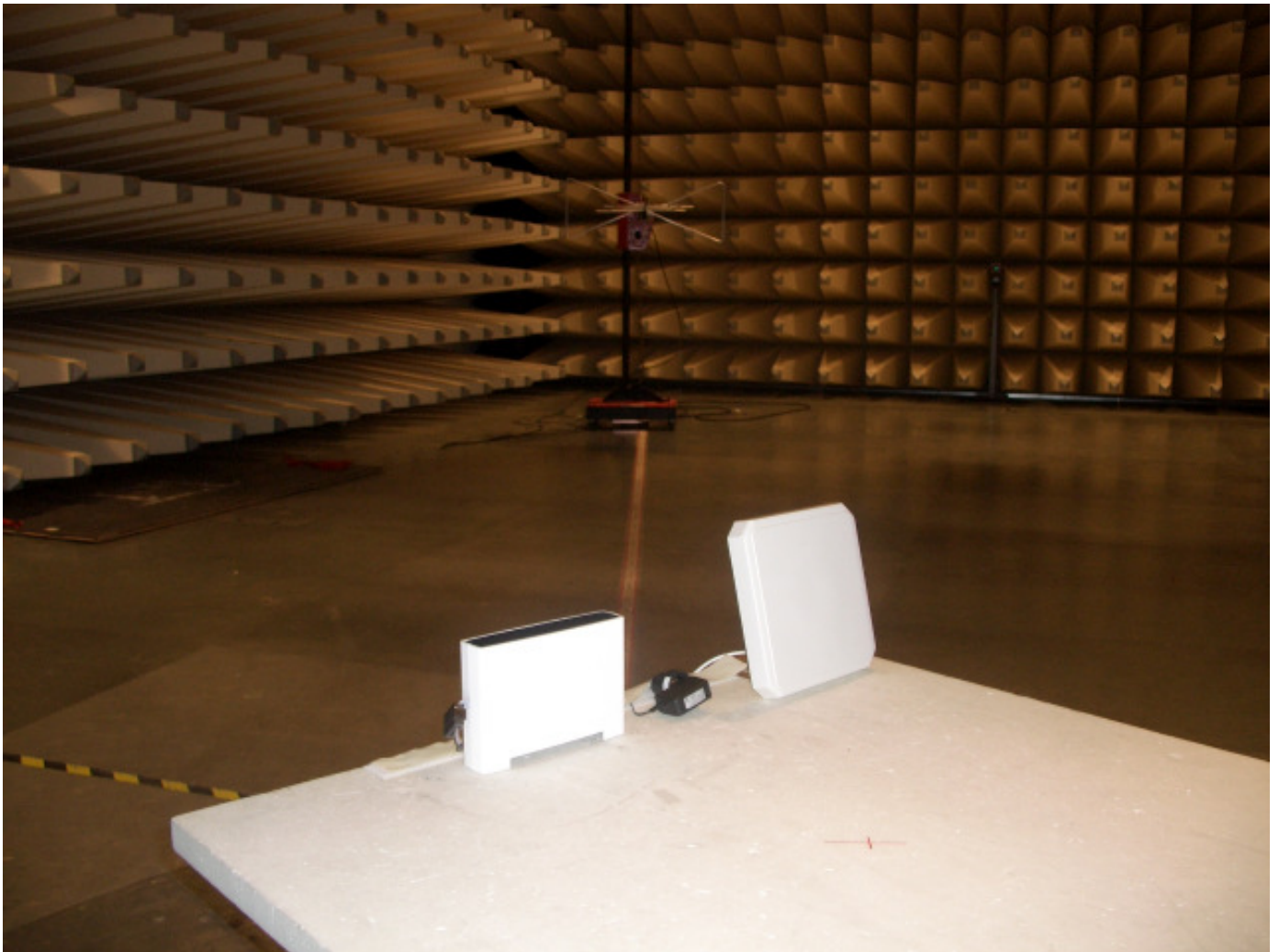
Anechoic chamber with 10m measurement distance
