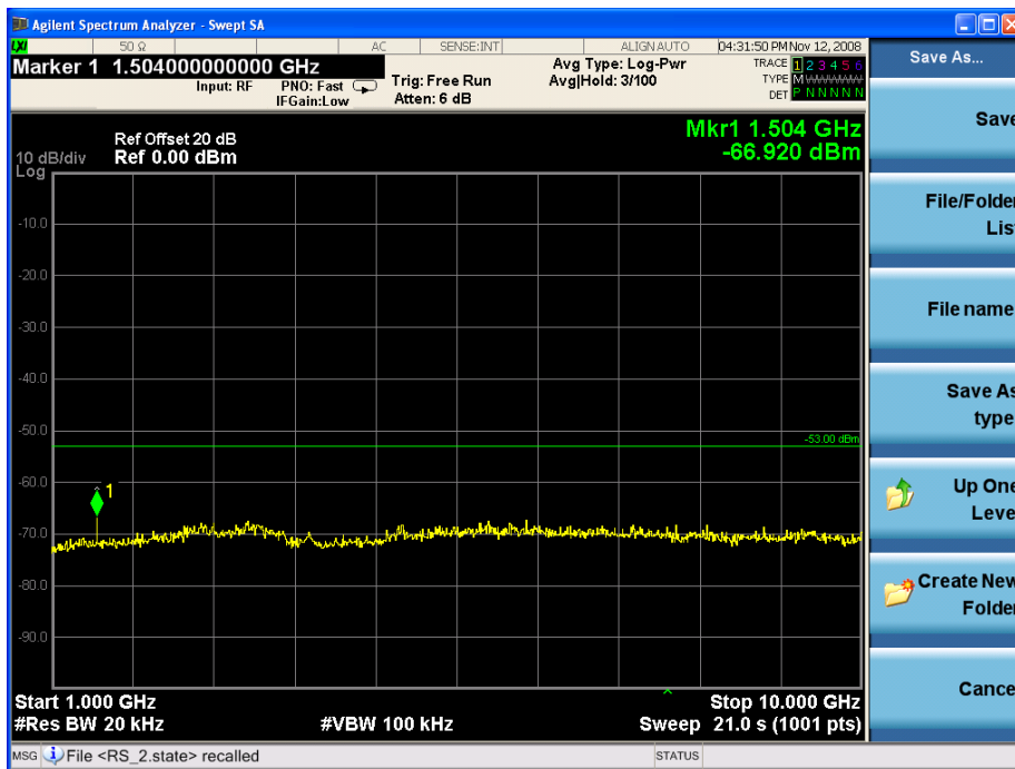
Receiver Spurious Emissions, Conducted, 1 GHz – 10 GHz
