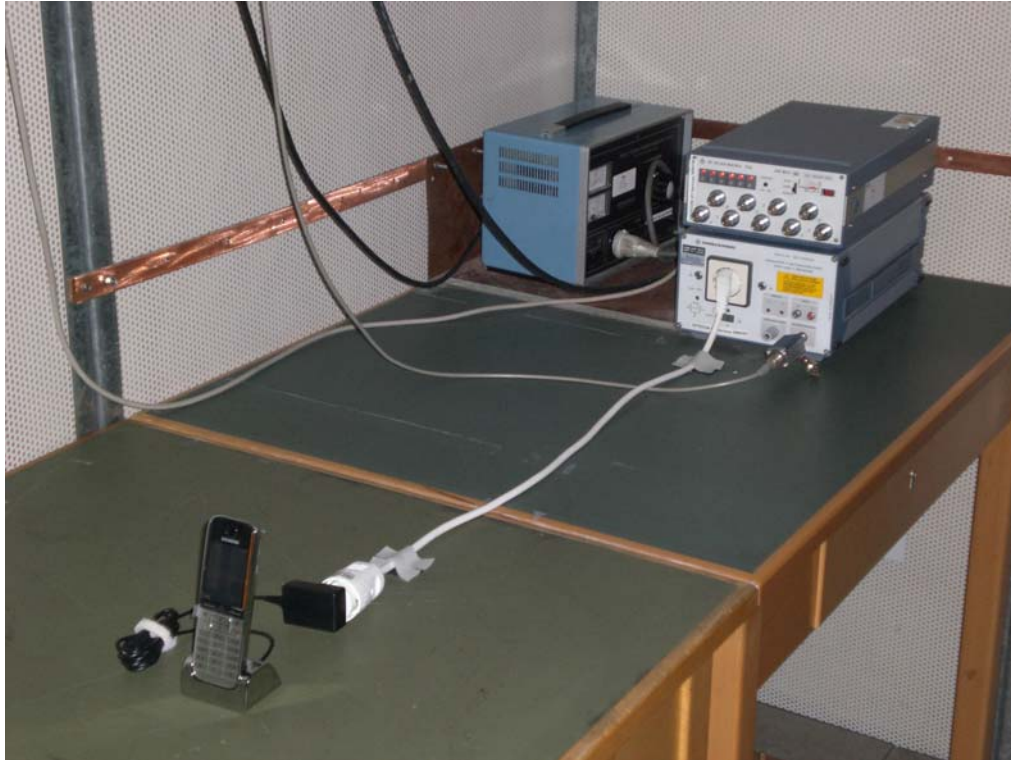
Photo 1: Power Line Conducted Emission Test
