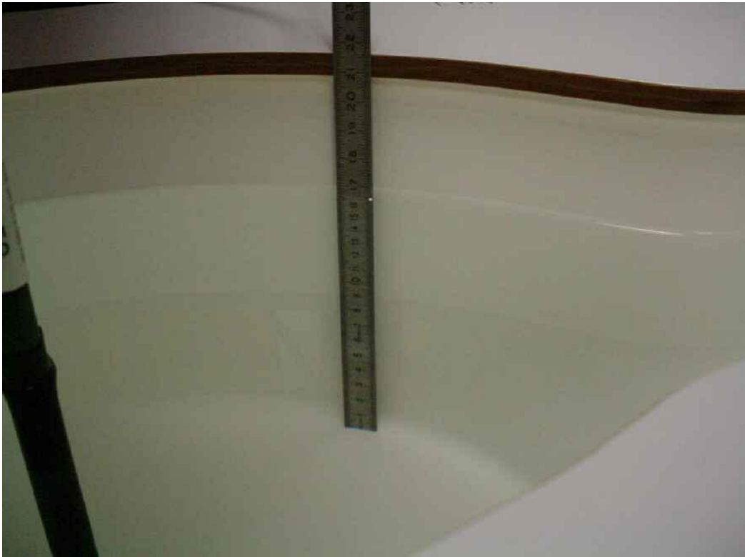
Photo 23: Liquid depth 1900 MHz body simulating liquid
