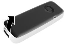
To **change the battery**, place your fingernail in the cavity in the casing and pull the battery upwards.
