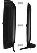
Place the cover in the notches on the back of the base station and click into place (not if mounting on the wall).
