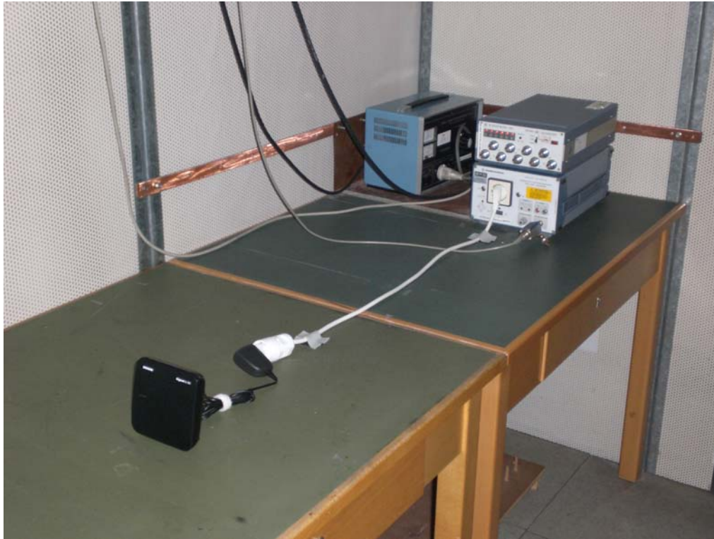
Photo 1: Power Line Conducted Emission Test
