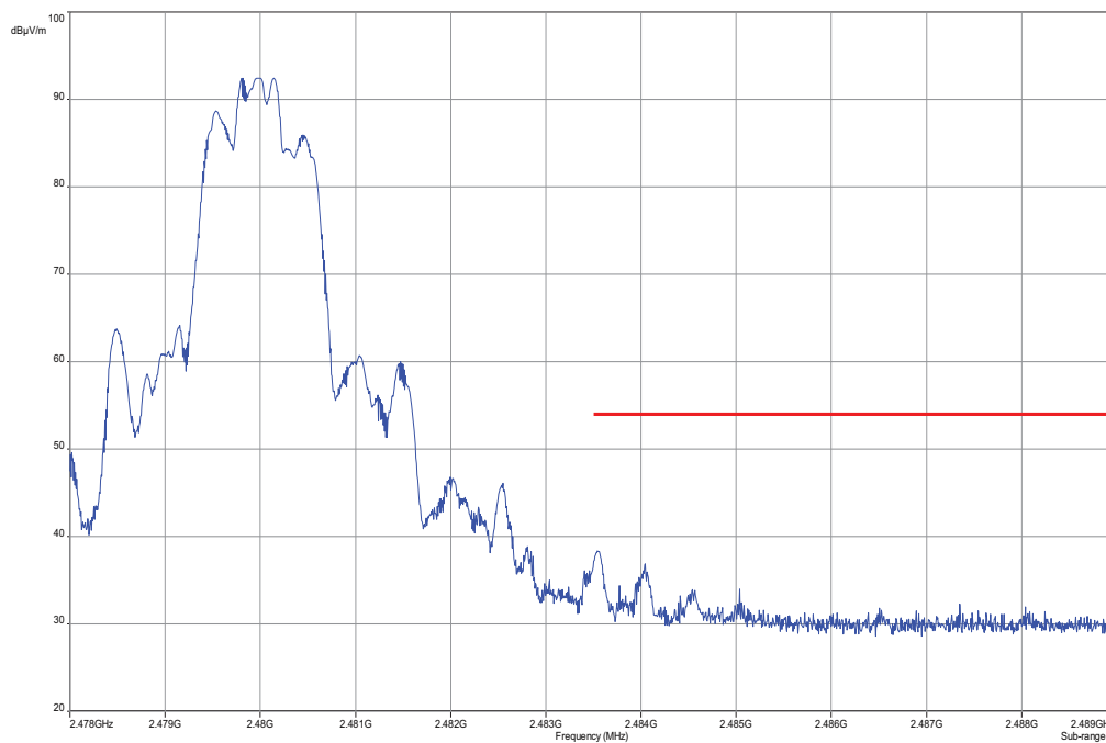
Plot 6: Upper band edge, 8 DPSK modulation, vertical & horizontal polarization
