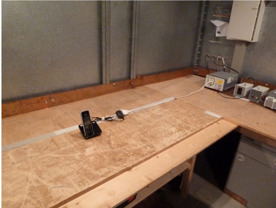
Photo 1: Power Line Conducted Emission Test
