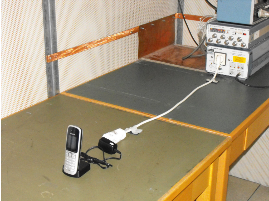
Photo 1: Power Line Conducted Emission Test
