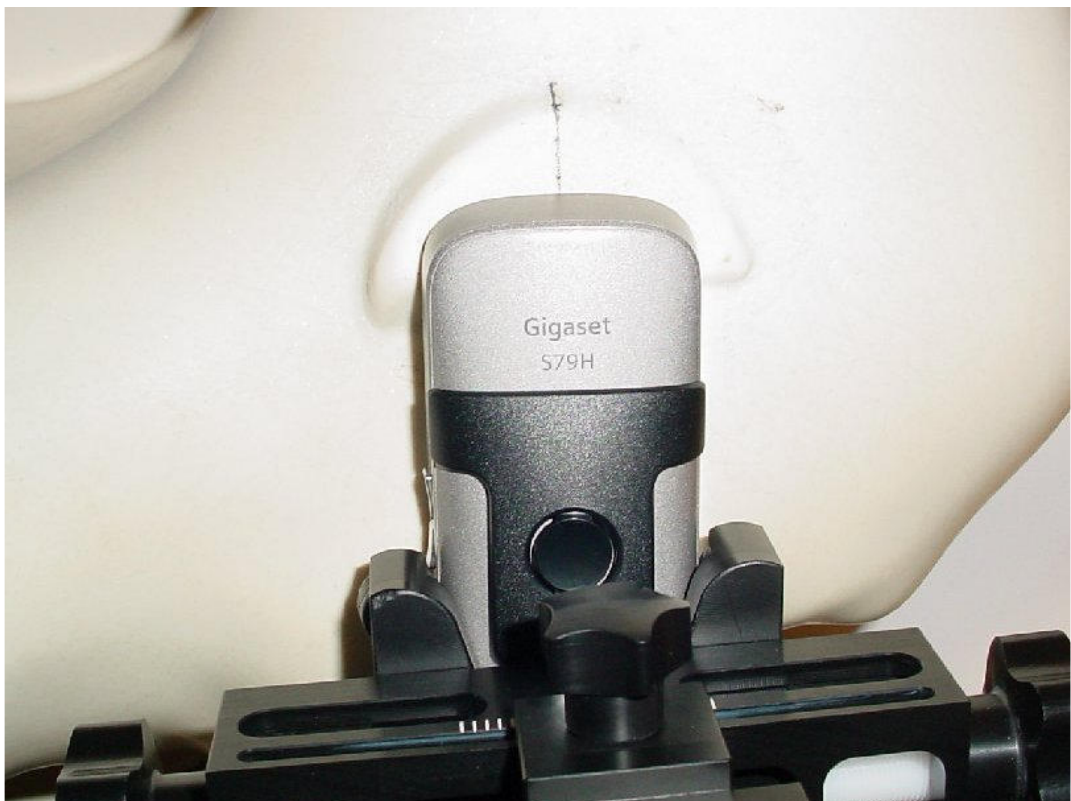
Photo 16: Test position right hand touched
