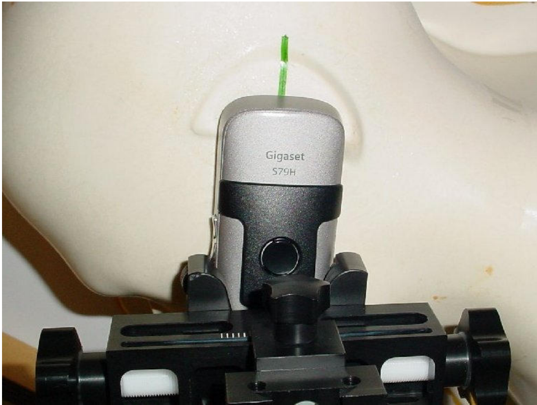
Photo 12: Test position left hand tilted 15°
