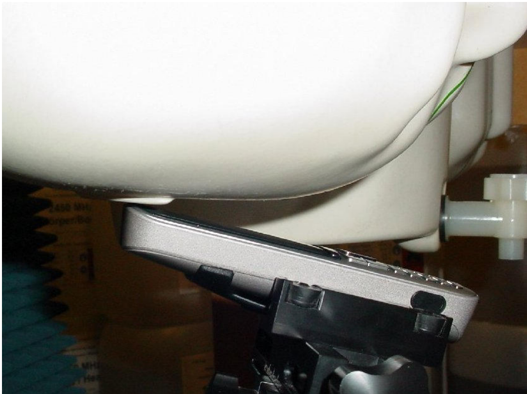
Photo 18: Test position right hand tilted 15°
