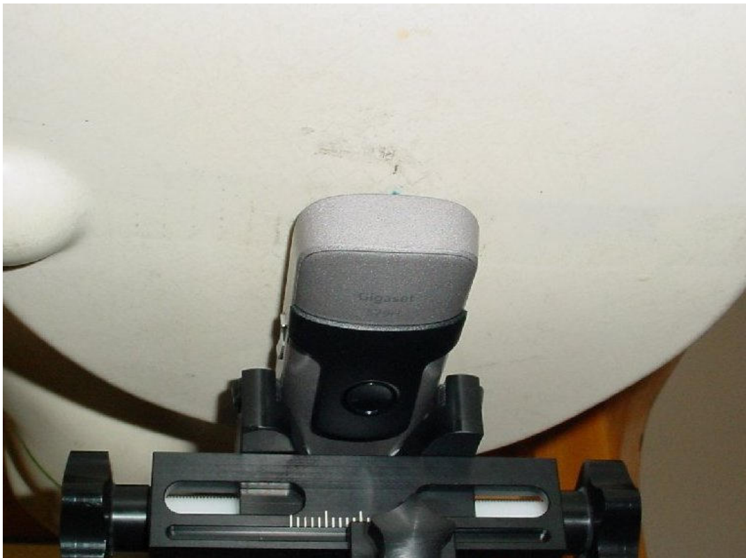
Photo 20: Test position body worn front side without any distance
