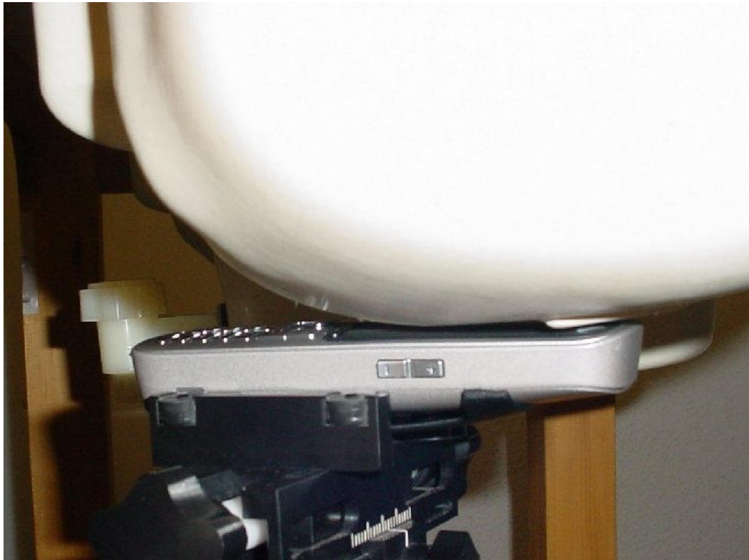
Photo 10: Test position left hand touched
