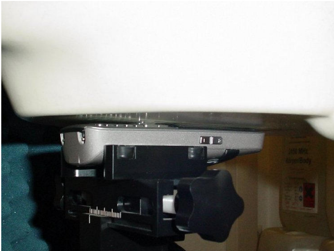
Photo 20: Test position body worn front side without any distance
