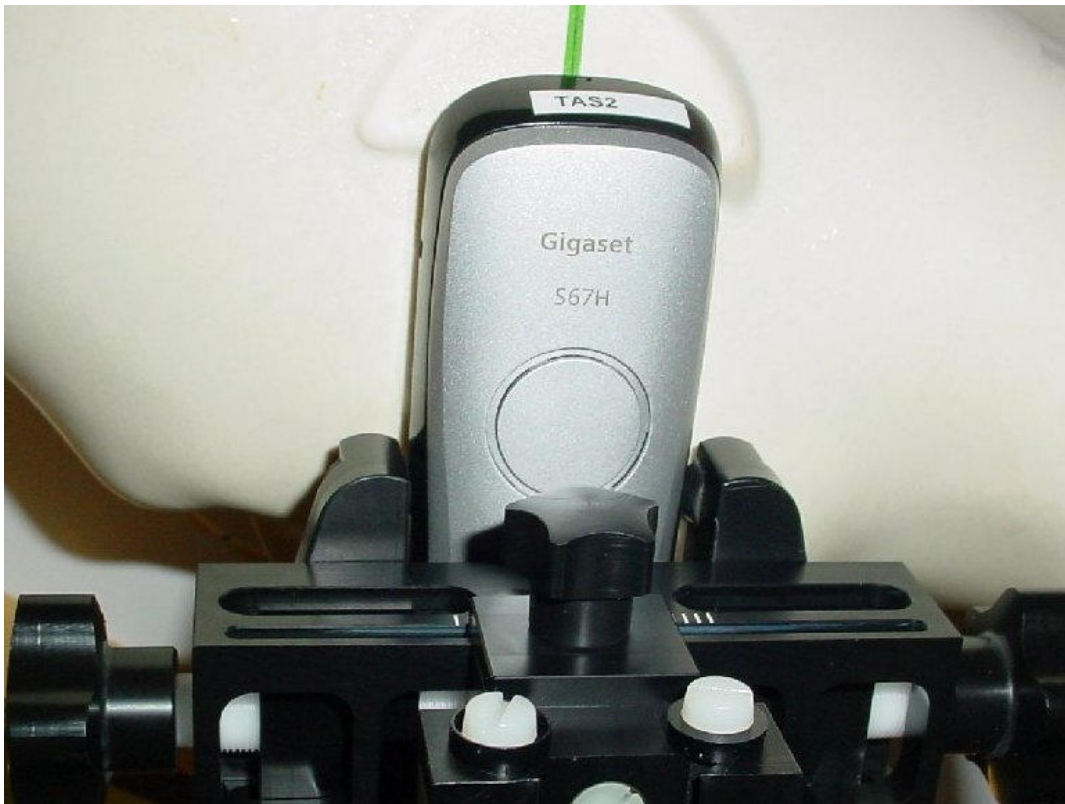
Photo 10: Test position left hand tilted 15°
