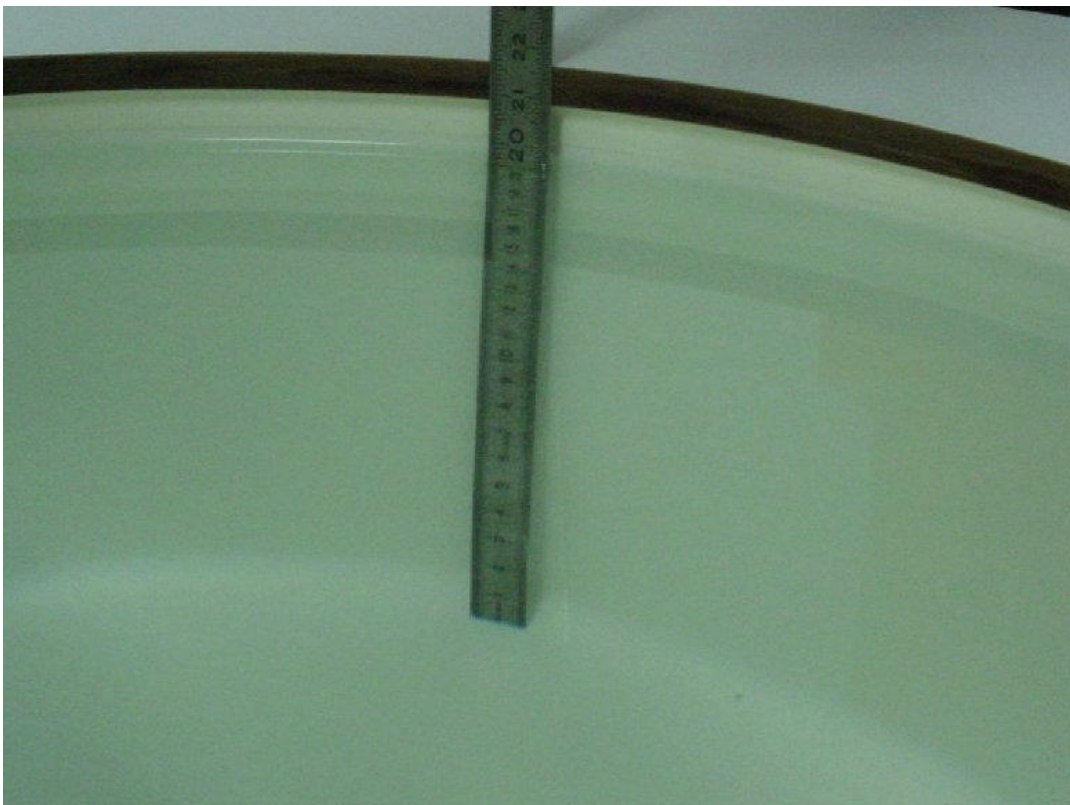
Photo 22: Liquid depth 1900 MHz body simulating liquid
