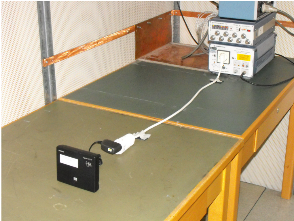
Photo 1: Power Line Conducted Emission Test
