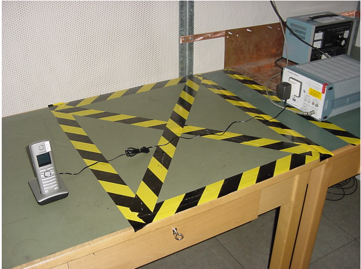
Photo 3: Conducted Emissions S45
