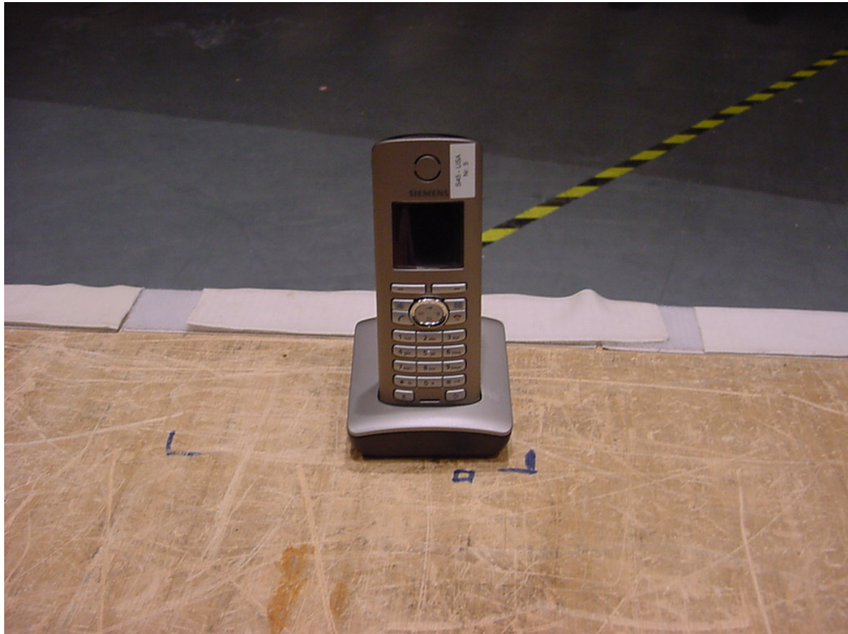
Photo 1: Radiated Emissions S45
