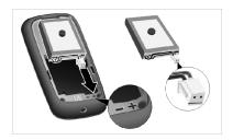
▶ Place the battery into the casing.
