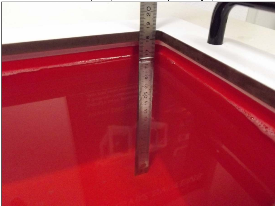
Photo 2: Liquid depth 1900 MHz body simulating liquid
