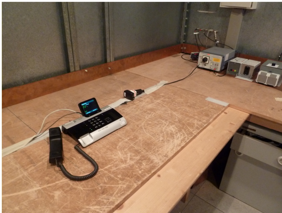
Photo 1: Power Line Conducted Emission Test
