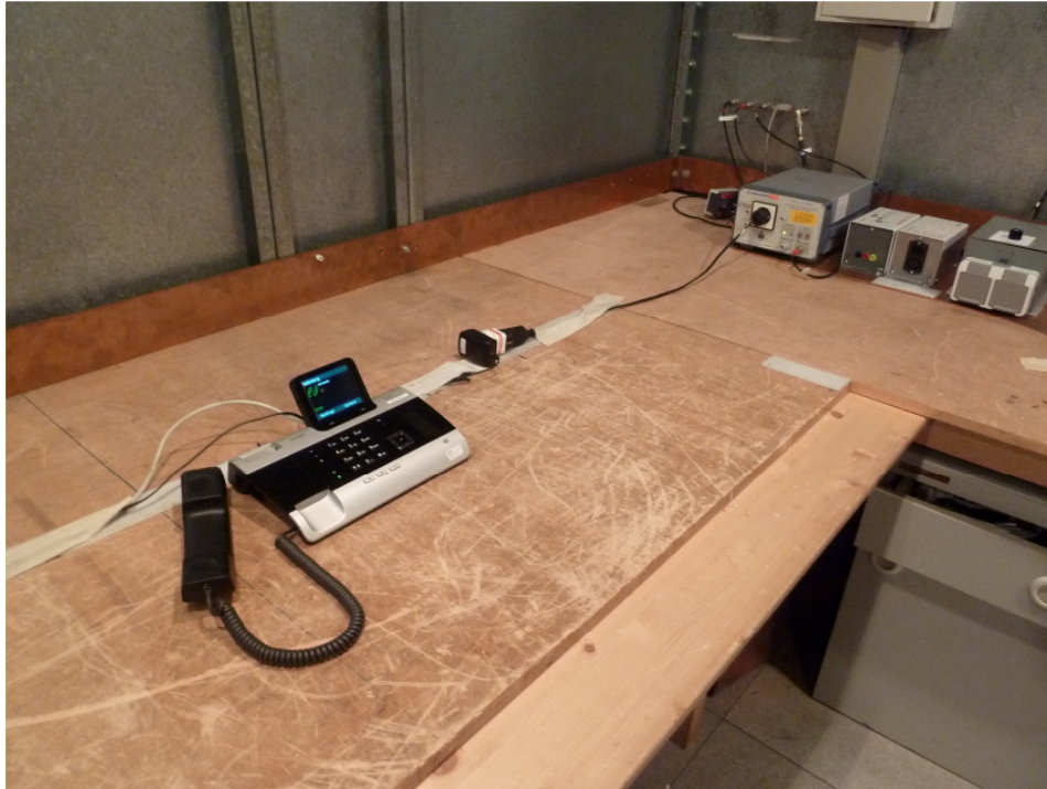
Photo 1: Power Line Conducted Emission Test
