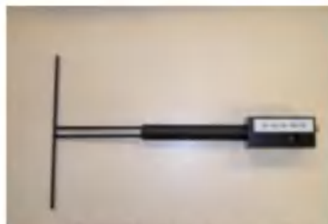
Figure 1 – Satimo COMOSAR Validation Dipole
