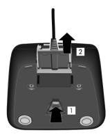
To disconnect the plug from the charger, press the release button **1** and disconnect the plug **2**.
