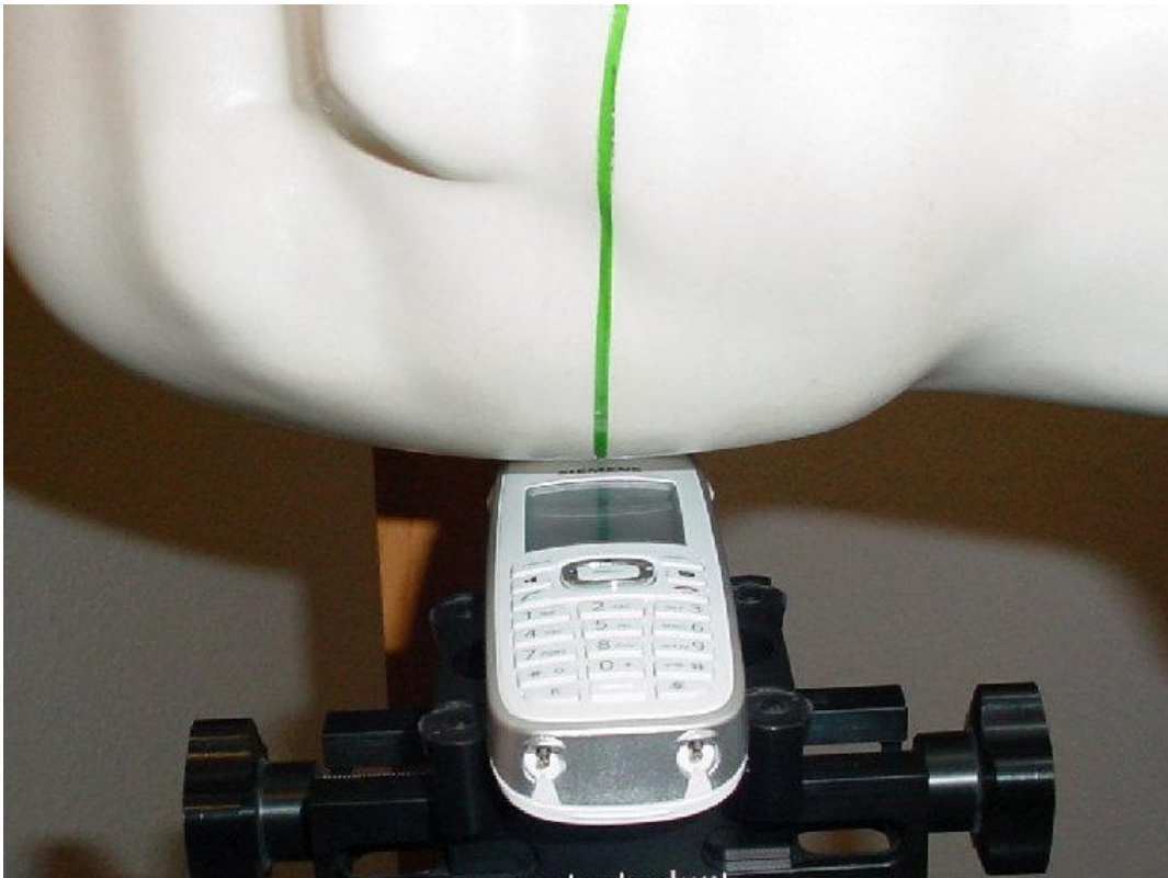
Photo 18: Test position right hand tilted 15°
