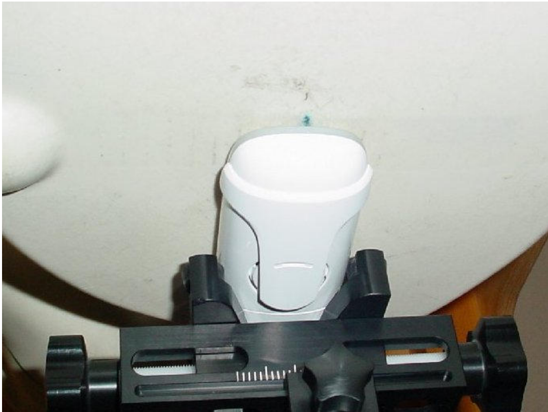
Photo 22: Test position body worn rear side without any distance
