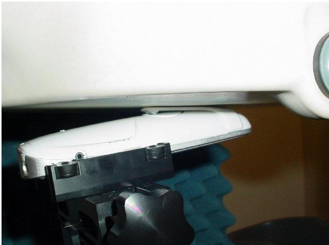
Photo 22: Test position body worn rear side without any distance
