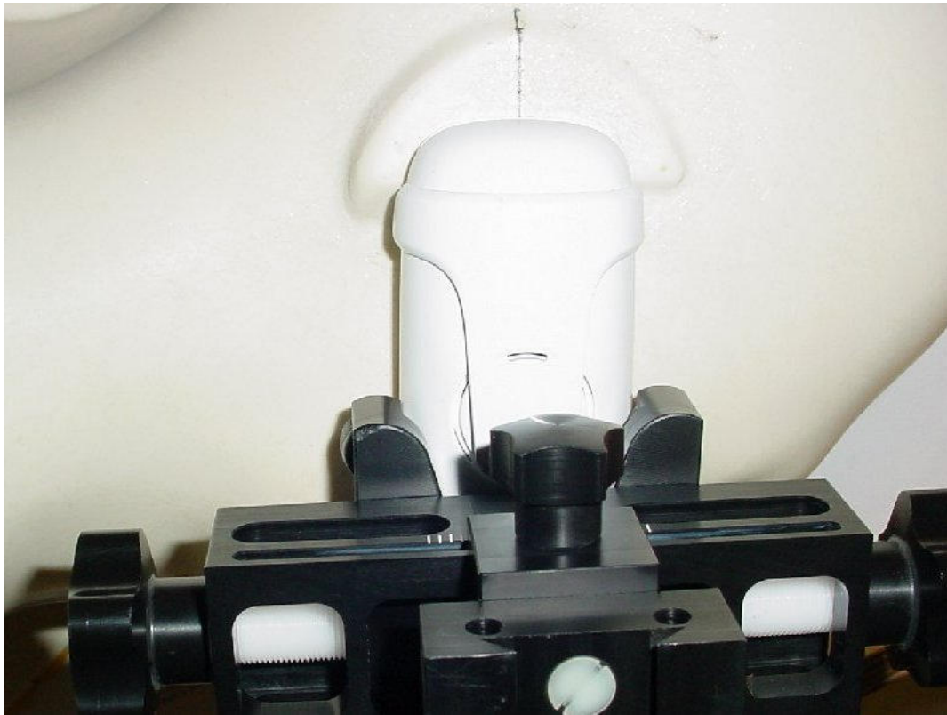
Photo 18: Test position right hand tilted 15°
