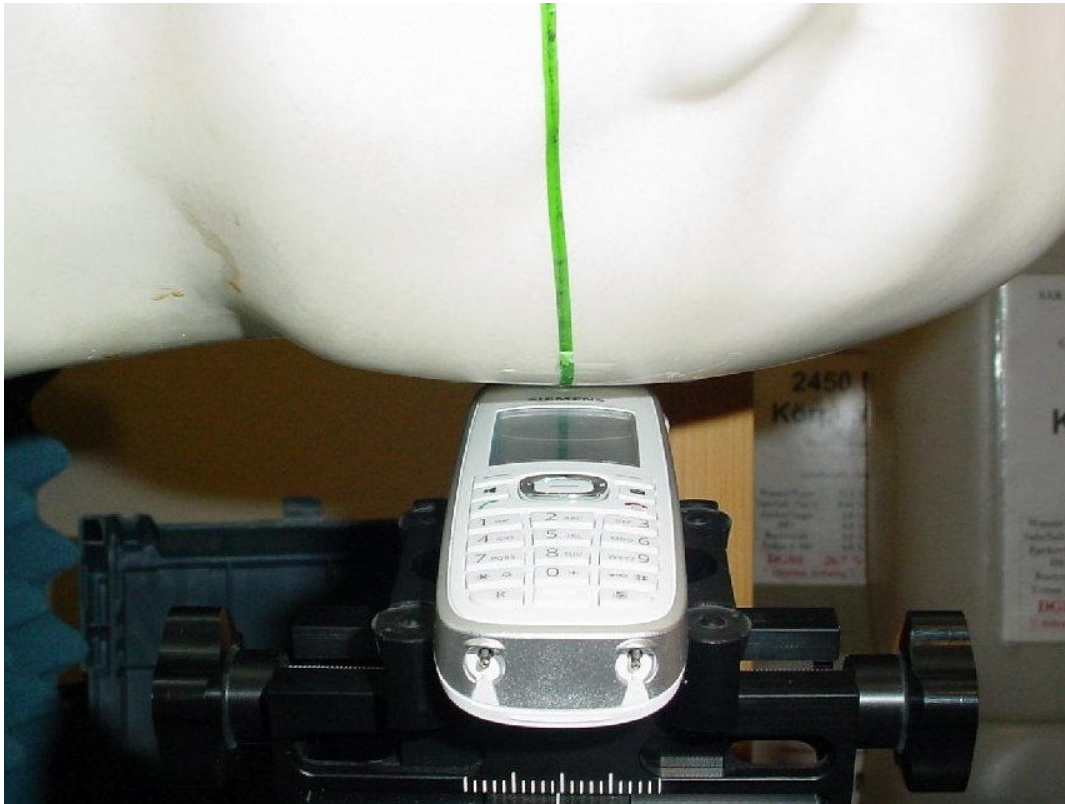
Photo 14: Test position left hand tilted 15°
