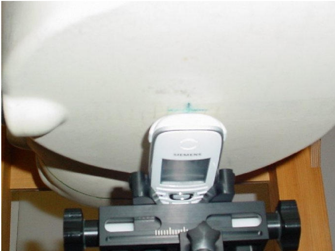
Photo 24: Test position body worn rear side without any distance and clip
