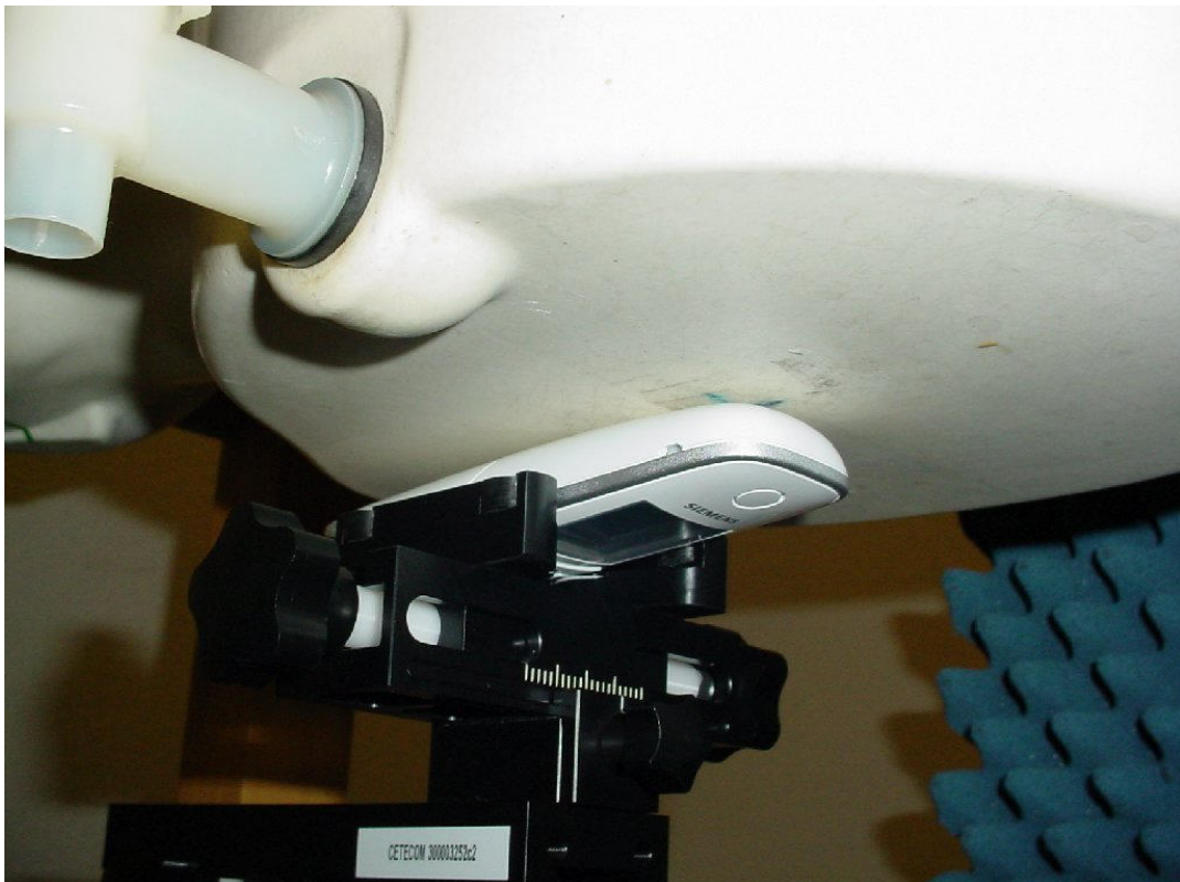
Photo 24: Test position body worn rear side without any distance and clip
