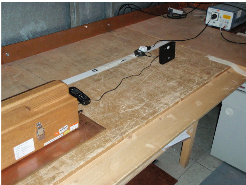
Photo 2: Power Line Conducted Emission Test
