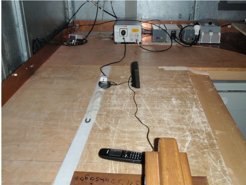
Photo 1: Power Line Conducted Emission Test
